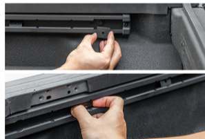
12. For the driver side installation, place three ⑩ into the slide rail.
